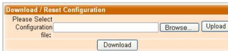
The screenshot shows a web interface for downloading or resetting configuration. The title is 'Download / Reset Configuration'. It features a text input field with the label 'Please Select Configuration file:' and two buttons to its right: 'Browse...' and 'Upload'. At the bottom of the interface is a 'Download' button.
